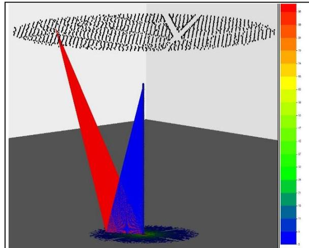
Figure 1: 3D VSP survey design for VSP #2 showing surface sources (black) and 3C borehole geophone array (blue). The estimated illumination at the deepest target depth at this location is shown along with the down-going direct rays (red) and up-going reflected rays (blue) for a single source.
