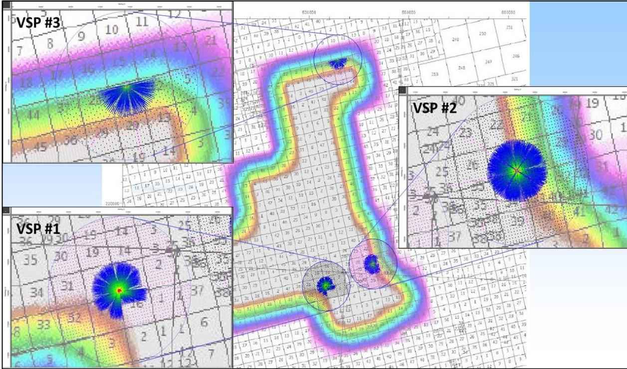
Figure 2: The locations of three 3D VSP surveys positioned within the larger 3D/3C surface seismic survey. Each location shows the estimated illumination at the deepest target depth along with the surface source locations. VSPs #2 and #3 recorded both P-wave and S-wave vibrator sources. VSP #3 was restricted to source locations south of the survey boundary.
