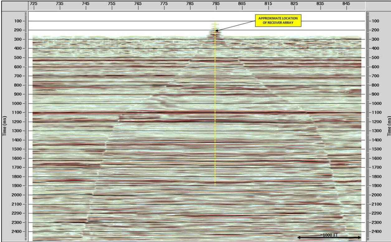
Figure 4: 3D P-wave reflection image for VSP #2 overlain on legacy 3D surface seismic survey. The approximate location of the total geophone array is shown in yellow. Differences in the start times are related to the final processing datum chosen for each project.
