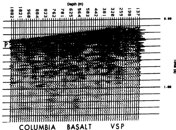
Figure 1. Vertical component of VSP through basalt.
