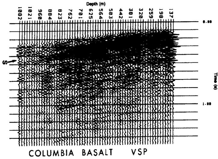
Figure 2. Horizontal component of VSP through basalt.
