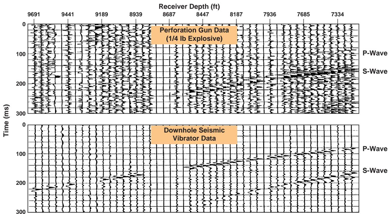
Figure 8. Comparison between data from a small explosive inside a perforation gun and data from the downhole vibrator. The survey was performed in east Texas. The data were recorded on a 48-level, cemented three-component receiver array.
