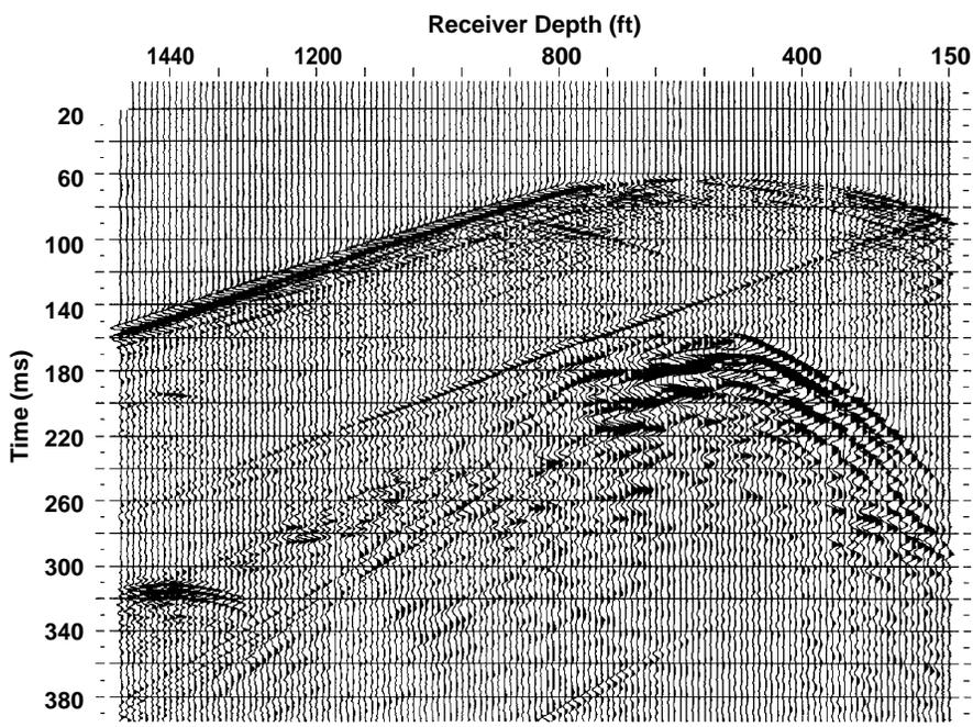
Figure 2. Common source fan showing direct  $P$ -wave and  $S$ -wave arrivals.
