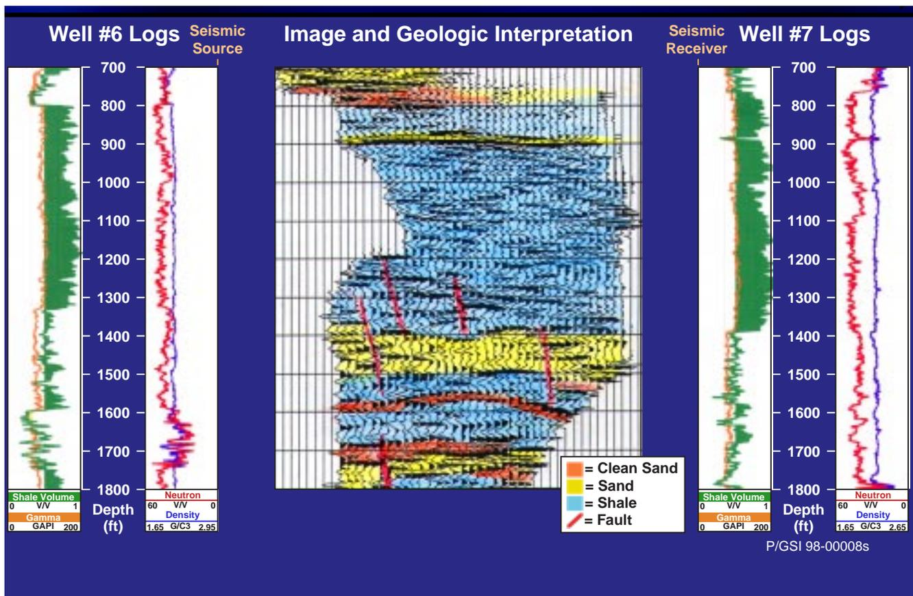
Figure 6. Interpreted crosswell seismic image with well logs on either side. The reflection image shows beds and fault displacements with resolution of a few feet.
