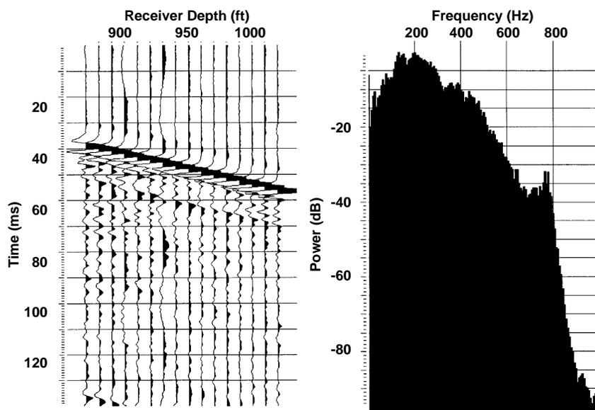
**Figure 4. Power spectra of direct *P*-wave arrival averaged over traces shown on left.**
