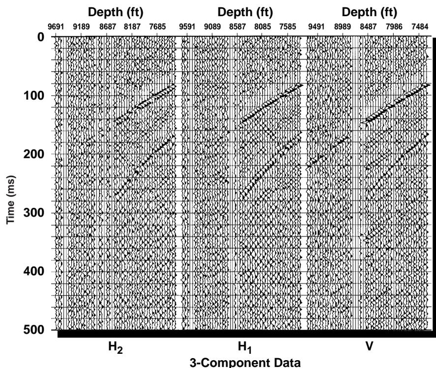
**Figure 10. Borehole seismic data recorded using the downhole vibrator and the cemented, three-component 48-level geophone array. All three components are shown. The shear-wave reflections from below the receiver array are especially apparent on the  $H_1$  component. The data are aliased since the spatial sampling of the array (50 ft) is approximately the same as the shortest wavelength (40-50 ft).**
