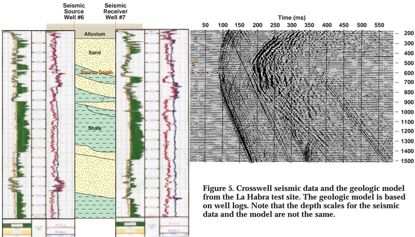
Figure 5. Crosswell seismic data and the geologic model from the La Habra test site. The geologic model is based on well logs. Note that the depth scales for the seismic data and the model are not the same.
