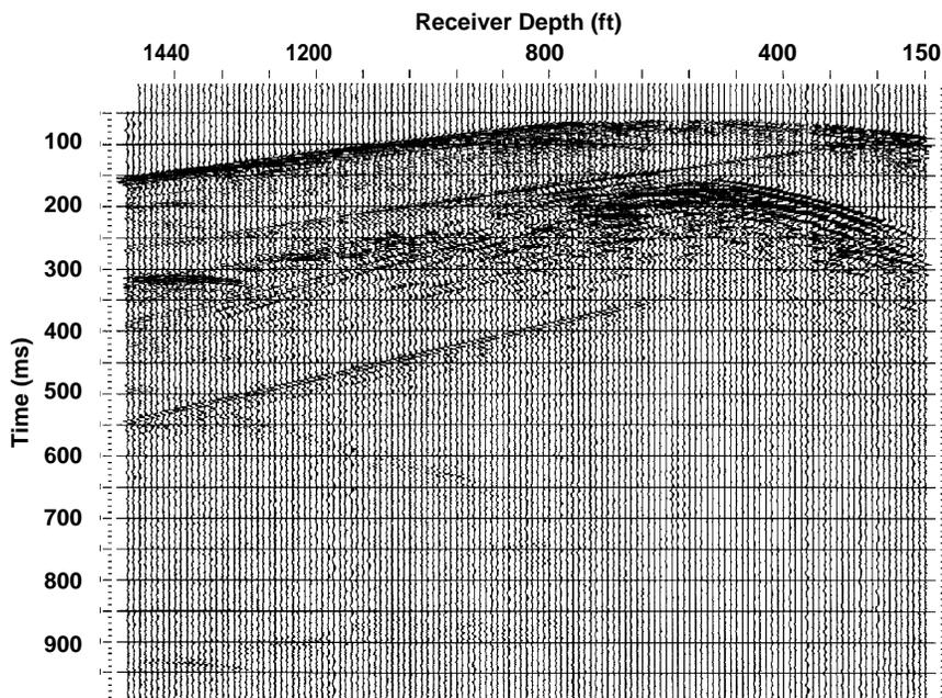
**Figure 3. Common source fan showing deep reflection intersecting left edge of plot at about 500 ms.**
