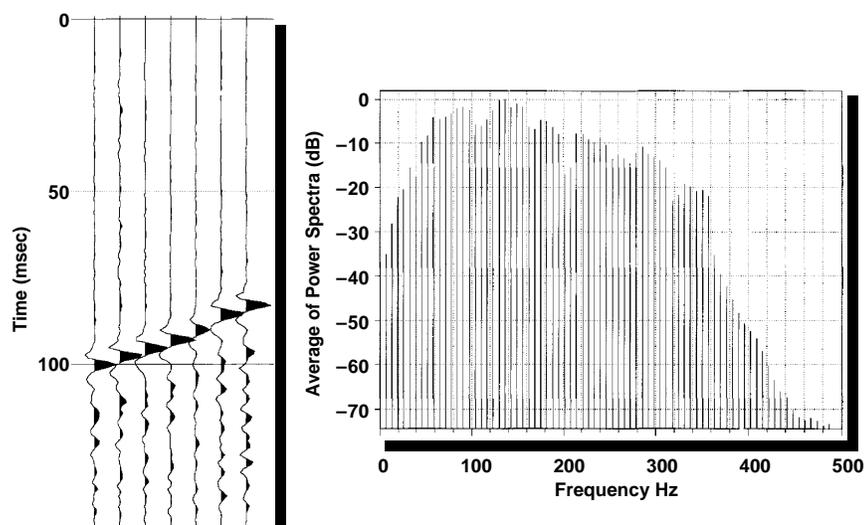
**Figure 9. Amplitude spectrum of data from the downhole vibrator. The distance between the source and receivers for the data exceeds 2000 ft.**
