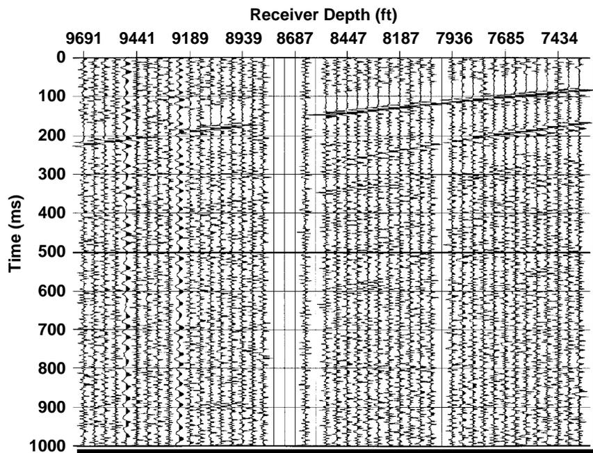
**Figure 11.** 1 s of the vertical component of the crosswell data. The longest direct travel path from the source (positioned at 6000 ft) to the deepest receiver (9691 ft) is 3900 ft. This arrival is seen at 220 ms on the far left of the record. Reflections from geologic interfaces at depths several thousand feet below the receiver array can also be seen. Some of these reflections can be seen at a travelttime of 1 s, indicating a total travel path in excess of 16 000 ft.
