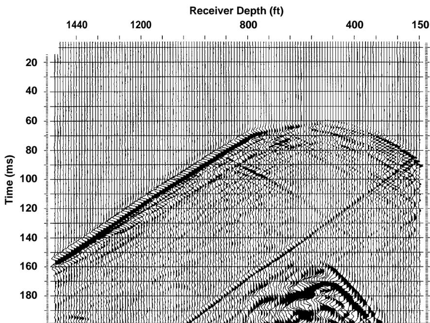
Figure 1. Common source fan. The source was positioned at a depth of 500 ft. The five-level receiver array was positioned from 150 to 1500 ft in 10-ft increments.
