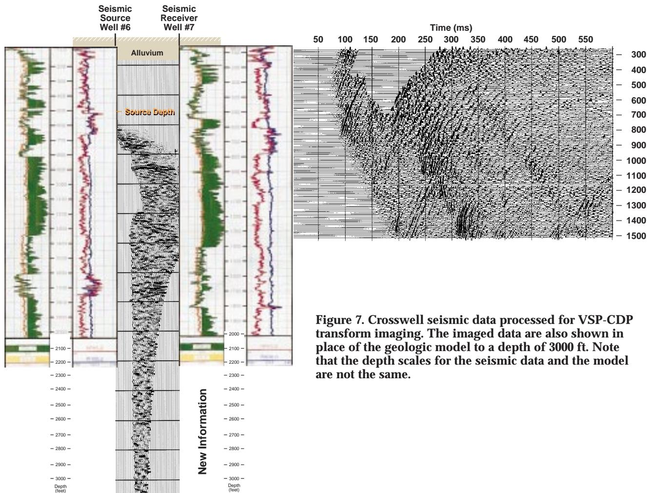
Figure 7. Crosswell seismic data processed for VSP-CDP transform imaging. The imaged data are also shown in place of the geologic model to a depth of 3000 ft. Note that the depth scales for the seismic data and the model are not the same.
