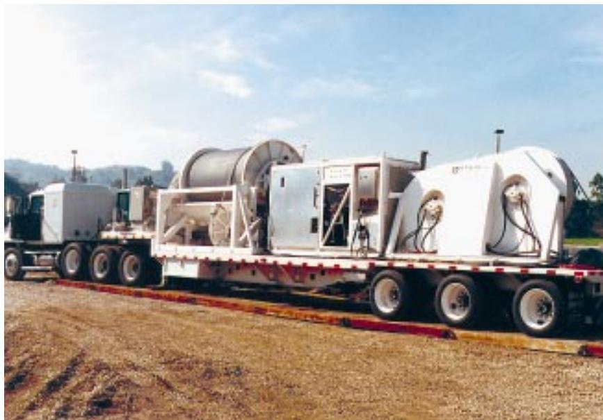
a five-level, clamped, three-component tool developed by Exxon Production Research. At the time of the first test, the receivers operated on a seven-conductor wireline. The system now operates on a fiber-optic wireline. The maximum number of receiver modules in the array is currently 10. The data-sampling interval is 0.25 ms.
