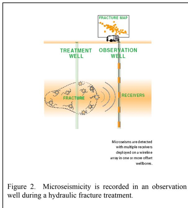
Figure 2. Microseismicity is recorded in an observation well during a hydraulic fracture treatment.
