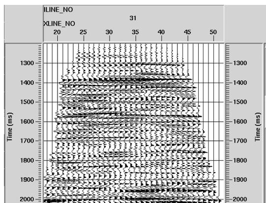
Figure 1. Vertical slice from full 3D VSP volume used in this study. Frequency content in the stacked image exceeded 140 Hz.
