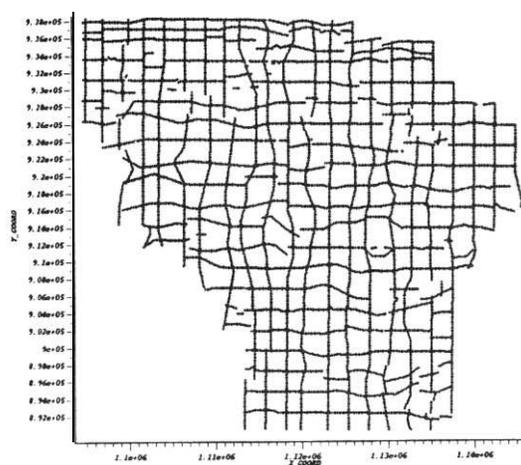
Figure 2. 3-D seismic survey area showing irregular source (E-W) and receiver (N-S) lines.
