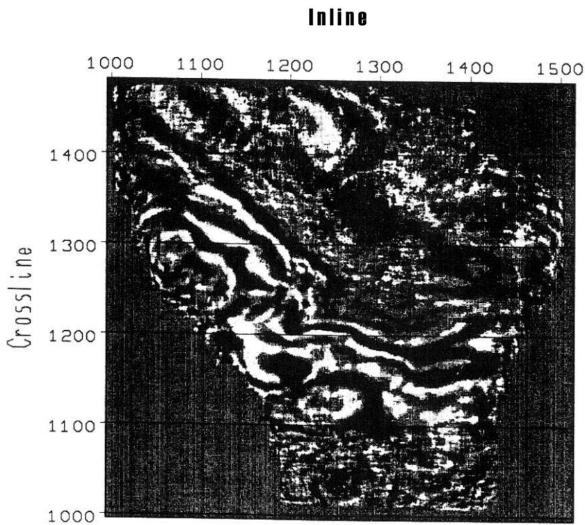
Figure 5. Time slice at 1920 ms extracted from 3-D migrated volume after applying optimized processing steps.
