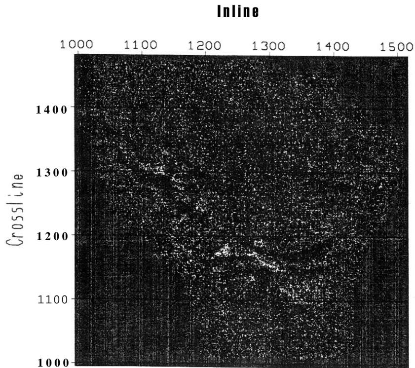
Figure 4. Time slice at 1920 ms extracted from 3-D stacked volume without optimized processing steps.
