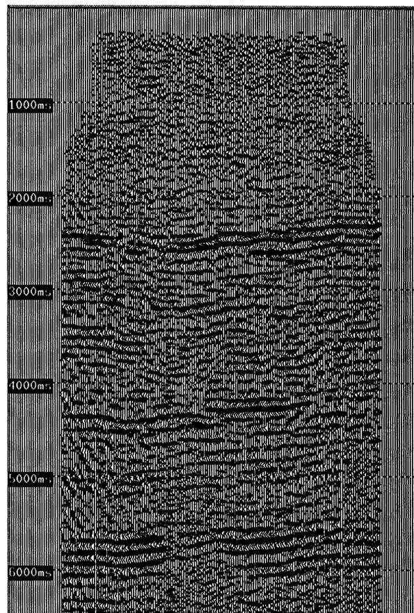
Figure 5. Final east-west stack with random noise attenuation and 8-24 Hz band-pass filter (H2 geophone, N90E/N270E azimuths).
