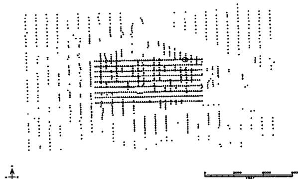
Figure 1. Surface source and receiver location map. Source lines are oriented north-south, receiver lines are oriented east-west. Source location for Figure 2 located in upper right corner of receiver patch denoted by an open circle. Map scale is approximately 1:120,000.
