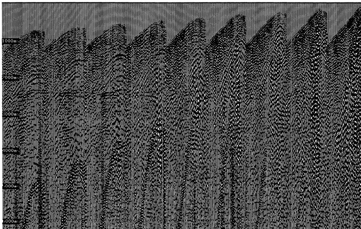
Figure 2. Typical shot record (H1 geophone). Note converted-wave reflections at 2.4 seconds.
