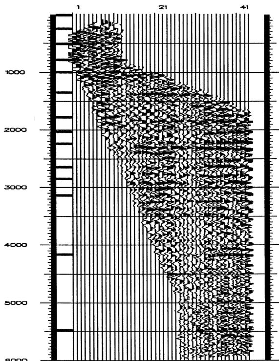
**Figure 3.** Common-conversion point supergather for the H1 geophone with statics, NMO, and mute applied. Trace spacing is 33 m and the propagation direction is N90E/N270E.
