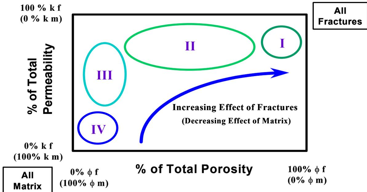
**Figure 1.** Reservoir classification (after Nelson, 2001) based on percent reservoir porosity and permeability in terms of percent due to matrix versus percent due to fractures. Type I reservoirs are heterogeneous and anisotropic, where fractures provide the essential reservoir porosity and permeability. At the other end of the spectrum, type IV reservoirs fractures provide no additional porosity or permeability but are still anisotropic and can create barriers.
