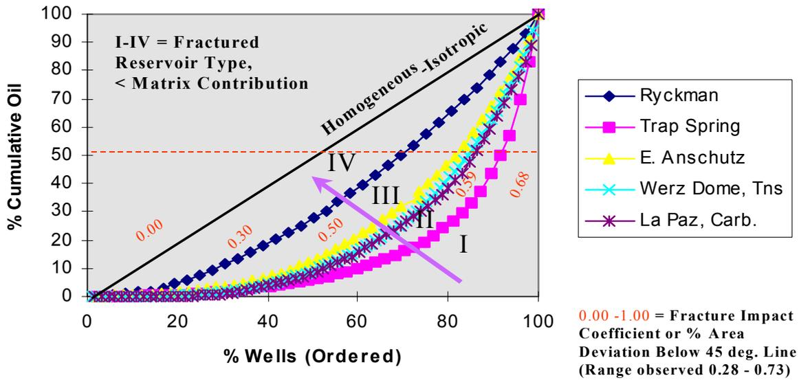
**Figure 2.** Percent cumulative oil versus percent wells (ordered from least to most productive) is cross-plotted for various fractured reservoirs along with reservoir type I through IV (after Nelson, 2001). Fracture impact coefficient is the percentage of the area below the homogenous-isotropic line, and provides a quantitative measure of increased production costs and *fracture denial*.
