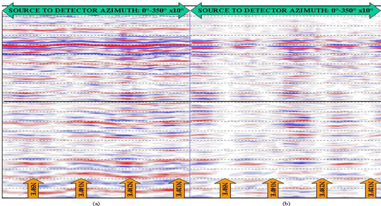
**Figure 2.** Azimuth-limited common-detector stack traces from detector location 1: a) radial and b) transverse component. Approximate principal S-wave directions at 50, 140, 230 and 320 degrees, as determined by locating the null transverse component traces, are shown as orange arrows. Note the polarity change across these null zones and that the directions are separated by 90 degrees.
