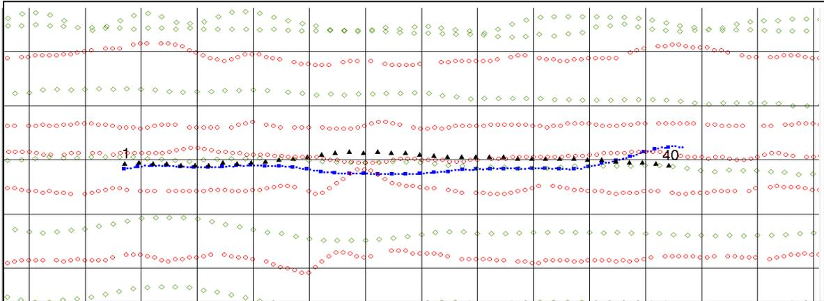
**Figure 1.** Map showing the source and detector locations for the 2002 survey (red source circles and black detector triangles) and the 2003 survey (green source diamonds and blue detector squares). Note that the 2002 survey used a 50 m detector spacing and 25 m source spacing while the 2003 used a 12.5 m detector spacing and 50 m source spacing. A blanket of sources (not all shown) was utilized providing wide azimuth coverage at each detector.
